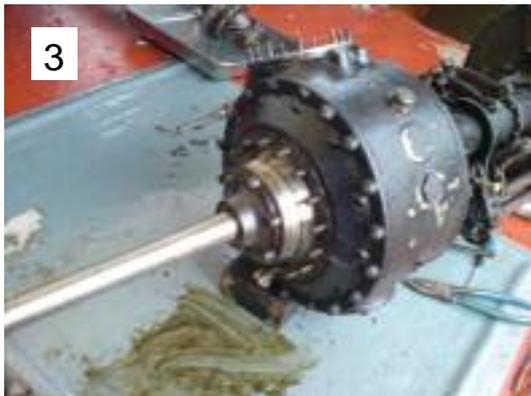
move the half shafts (not as easy as it sounds; this car is cleverly designed). At the top of the picture lies the pinion (I have replaced the two bearings, one is a double roller bearing) in that assembly (another two special tools made to do this). One of the oil seals is shown in its housing on the left side of the casing: 3
