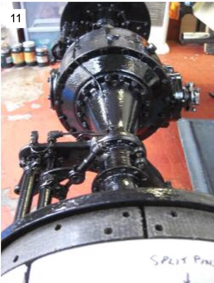
Underneath is the offside rear jack which is clamped to the spring 'U' bolts, ready for a lick of paint. The split pins had to be drilled out of the 'U' bolts and the threads cleaned up with a die nut. I also run a tap through the castle headed nuts (I think I need my floor re-painting!)
