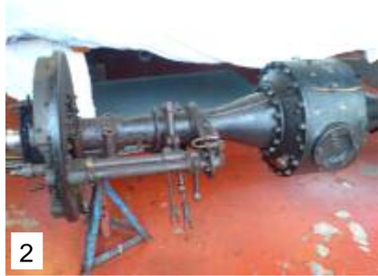
I was now able to remove the two axle tubes from the differential housing, then remove the two side plates from the centre housing and commence stripping the crown wheel assembly to re-
