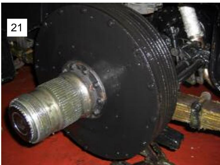
the drums without the need of the brake shoe cutter, by giving the shoes a slight dressing and remove any high spots: 21
