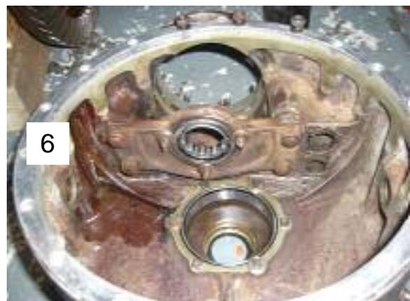
Picture 6 shows the differential casing with the bearings replaced, I replaced all the bearings and the two inner half shaft bushes while I had
