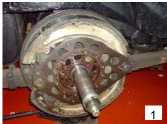
You can now see the axle placed on smaller axle stands ready to strip down. The brake backplate assembly on the left of the picture shows the hand brake shoes before removal and the brake cam shafts. The back plate is on a spline and if it had not been so seized the whole assembly could have been slid off the axle complete with the brake cam shafts. This would have given me access to the U bolt nuts and would
