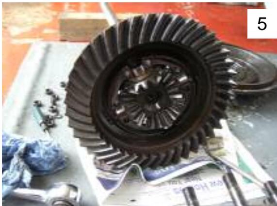
Now the crown wheel and planetary wheels are exposed with one half shaft removed ready for cleaning and inspection: 5
