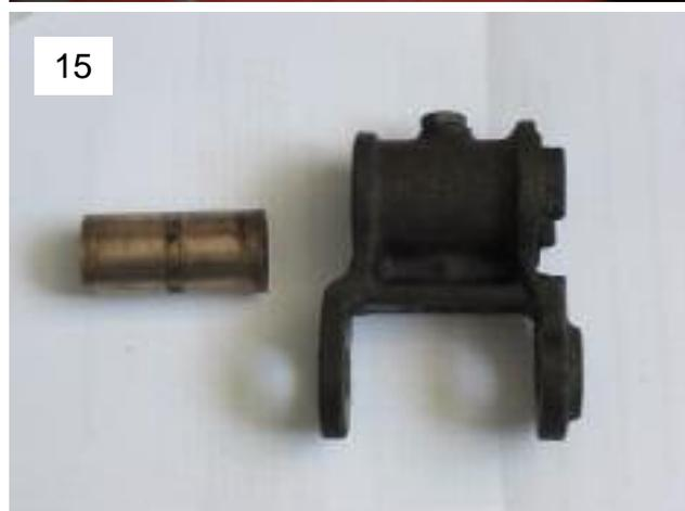
The spring hangers on both sides were removed and the top bushes replaced. The pins showed signs of wear, but because of the amount of work required to remove these pins, i.e. body off and possible heat required to release the tapers of the inner side of the pins, I decided instead to dress and grease the pins: 15
